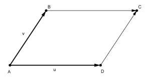
Note that the norm of the vector  $u \times v$ , that is  $||u \times v||$ , is equal to the area of parallelogram ABCD given by vectors u and v.
